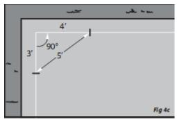
Note: These instructions assume the adjacent walls and support structures are square. In the event non-square walls result in very thin cut-strips at the edge of the layout, move entire layout in a direction that allows cut pieces to be a minimum (cosmetically and structurally) acceptable size. The minimum acceptable size is 6" inches.
