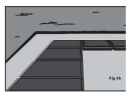
Note: Glue can be applied to the entire row of male locks to speed installation.
