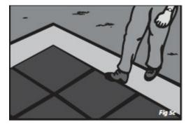
Note: Attention must be given to the amount of force used to align the tiles. Too much force will put the installation out of alignment.
