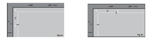
**b)** Measure 4 feet (or 8 feet) down the perpendicular string line and make a mark (Fig 4b - Line a-c).
