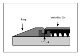
Note: The tile installer must determine the placement of the first row of tile so that the locking mechanism on the tile is utilized.
