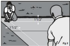
Note: Prior to beginning installation it is important to ensure that the string line is square. Ensuring that the string line is square will provide a smooth and neat installation. In order to check for square we will be using what is often referred to as the "three-four-five" (or "six- eight-ten") method.
