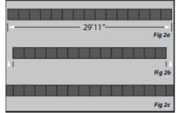
By increasing the perimeter cuts from  $\frac{1}{2}$ " to 1'  $\frac{1}{2}$ " we create a more visually attractive installation (Fig 2c).
