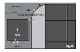
Note: Continue this process until enough references points have been transferred onto the tile. Straight regular cuts may only require two measurements per tile however irregular perimeters such as circles will require measurements in 2 or 3 inch increments across the tile. You can slide the square along the curve and get a reading of 'a and b' of pin point any location along the curve (Fig 6c).
