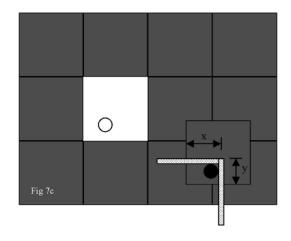
**5.** Place your template into the center of the "square" and mark the perimeter of the template. You are now ready to make your cut (Fig 7c).
