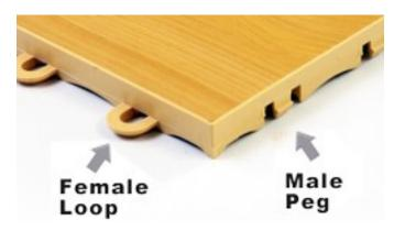
Step 2 Start by laying your first panel in any corner (male edges required) or garage opening (female edges required) roughly 1" from the wall. The loops should be pointed in the direction you want to add panels:
