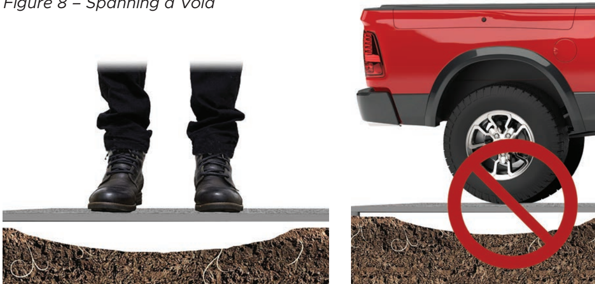
Figure 8 – Spanning a Void
