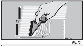
Note: The adhesive placed under keystone and strategic tiles must cure before compressive forces are applied.
