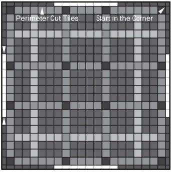
Cut tiles with a razor blade knife and metal straight edge on the line but with a back-cut or under-cut of approximately 5 degrees Install the cut tiles all the way around the perimeter. Start at the corners and work around (*Fig. 11*).
