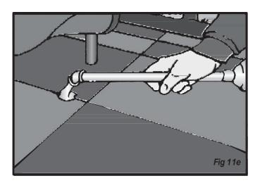
For most decks you can use a modified extension on the glue gun as shown in *Fig 11e*.
