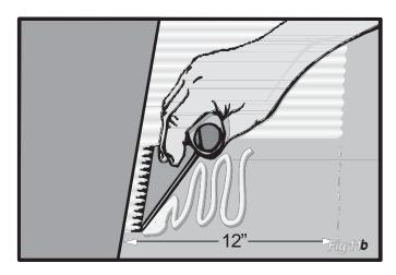
Ramp perimeter edging is adhered to the subsurface using the perimeter to sub-surfaces adhesive supplied with the order.
