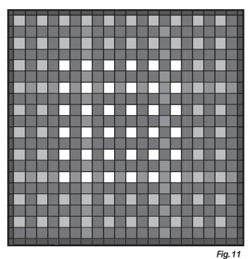
Compress tiles throughout the remainder of the area based on how the tiles are shifting during installation.
