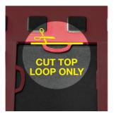
Trimming required of top loop/tab on the regular tiles where the Expansion Joint meets them.
