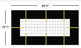
We recommend Expansion Joint strips be placed every 5' to 7' feet depending on exposure to direct sunlight. Length of the strip is dependent upon the sunlight exposure to that section. A minimum of 3' to 4' feet deep is recommended.
